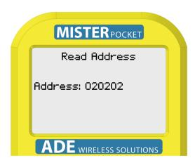
This function copies the address of the connected sensors to the memory of Mr Pocket.
