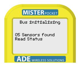
If you want to display all sensors connected to the bus with Mister Pocket (4.1.3), initialisation must first take place. The device then determines which and how many devices are present.
