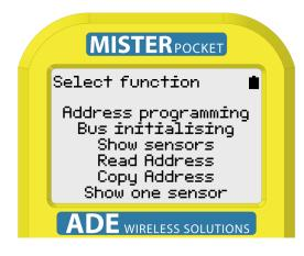
You can access the following functions for the optical sensor from this menu.
