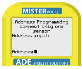
Every sensor must have a clear long address to ensure they can be differentiated in the bus system.
