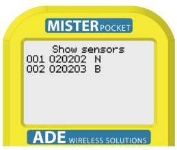
Before you can display the sensors in the bus, the bus has to be initialised (4.1.2).
