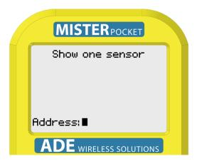
In order to be able to find a particular sensor in a shelf system, you can make the sensor flash with this function.
